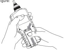
b. Insert a 9V battery into battery compartment, note the battery polarity, and then close the battery door, as shown in following figure:
