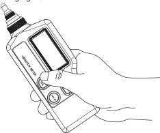
b. After the entire screen displays for 1 second, the default state is acceleration mode, if on the LCD displays the symbol or , please promptly replace the battery, as shown in following figure:
